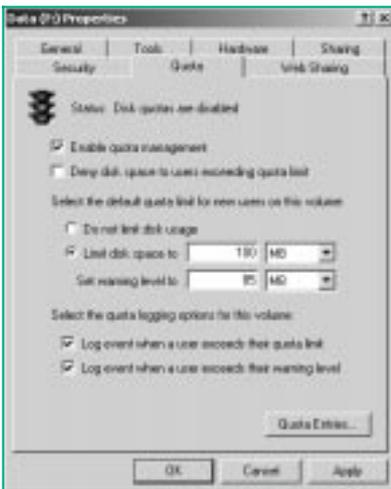
Figure 1 - Volume Properties window on a server before ena-
