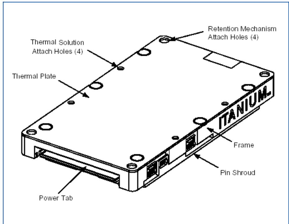
Figure 5 - Top view of the PAC418 Cartridge.
