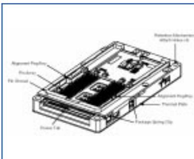
Figure 6 - Bottom view of the PAC418 Cartridge.
