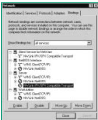
*Figure 1 - Disabling MS client bindings to IPX on Windows NT.*
