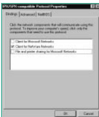
*Figure 2 - Disabling MS client bindings to IPX on Windows 95.*
